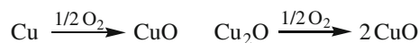
Scheme 3 Reactions involved in the third step of thermal decomposition of \text{CuAc}_2 \cdot \text{H}_2\text{O} in air
